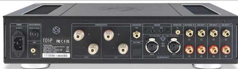
ABOVE: The one balanced XLR/three RCA line inputs are joined by an MM phono input (with separate earth), subwoofer output and a pair of 4mm speaker cable posts. The '+ve' and '-ve' outputs are floating so must never be connected to ground
